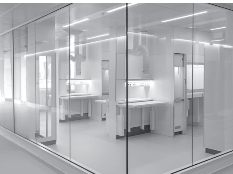
height adjustable workstations in Zystm 5 with local point extract to worktop
