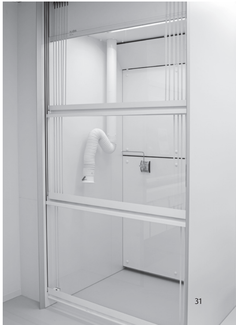
wall mounted extraction arm.
